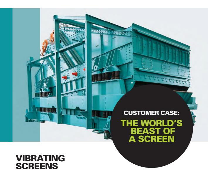
Meet the BEAST - at over 72 tonne in body mass, using twin exciter beams, four onemega newton force exciters and processing around 10,000 t/hr of slurry in a metal's extraction process, our BEAST Vibrating Screen, may well be the largest ever built.
