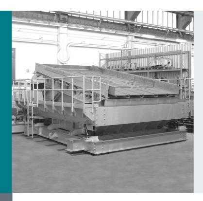
Classifying of hot bulk materials with a temperature of 300 °C ... 950 °C such as:
