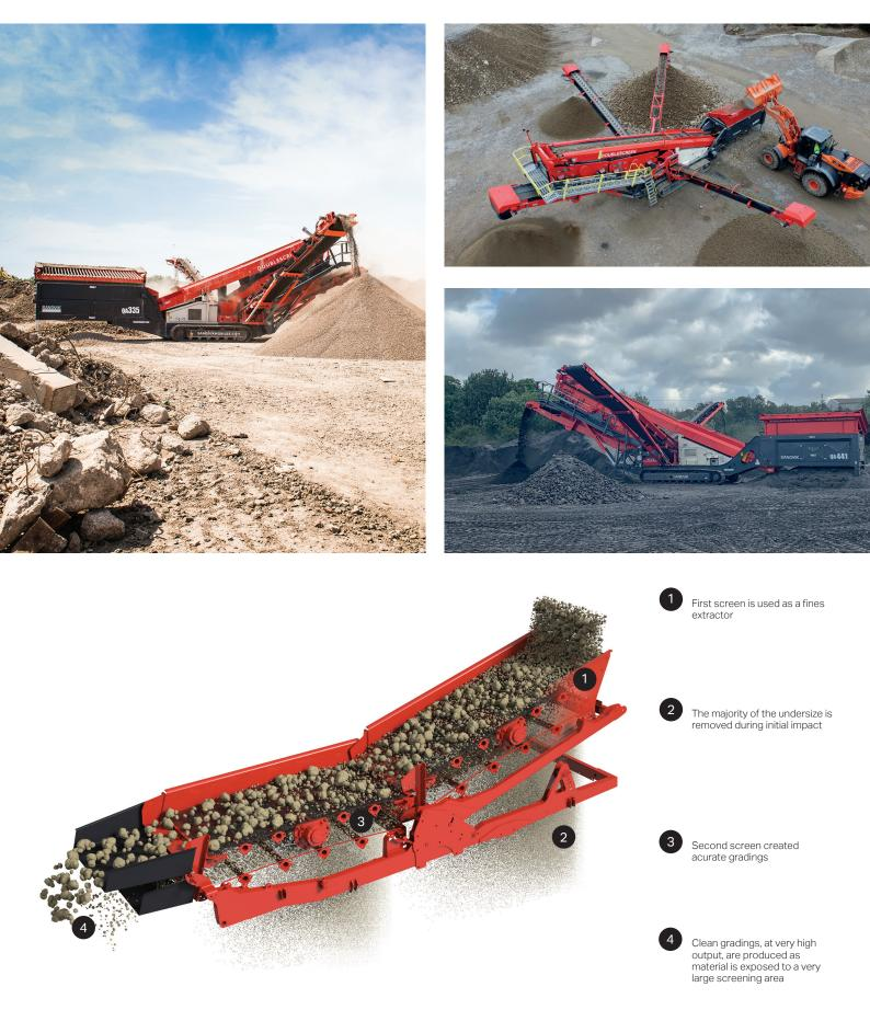
Sandvik's renowned Doublescreen box, features two independent double deck screen boxes. The primary screen works as a fines extractor, whilst the secondary screen operates as a grader.
