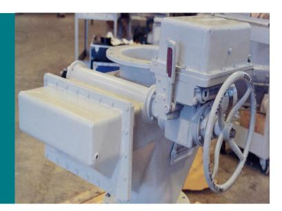
The Stock® Air Coal Valve (ACV) is a double rack and pinion style valve used as a means of isolation below a feeder. The airtight body provides positive shut-off to minimize hot air and gases from entering the feeder during maintenance. This is accomplished by means of a precision machined gate and inlet surface. The gate is supported on adjustable slide bars located between the gate surface and inlet skirt.
