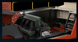
Includes integrated lifting jib, chain hoist and lifting cradle for safe removal, rotation and fitment of hammers
