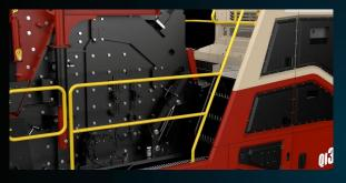
Emergency stop buttons and conveyor pull stop cords around the plant for easy access during operation
