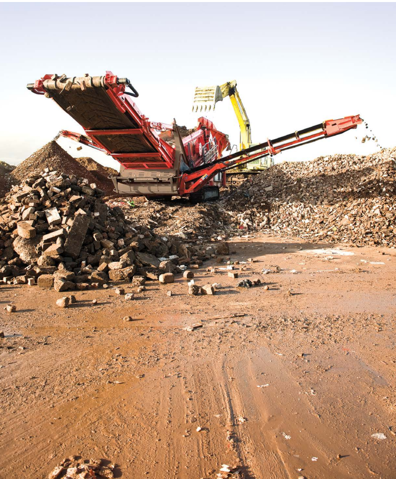
Ability to configure with punch plate, grizzly fingers, bofar bars, mesh or cascade fingers
