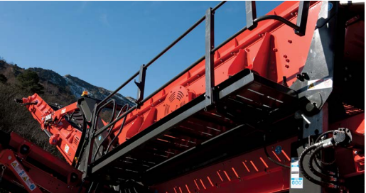
Hydraulically folding maintenance platforms
