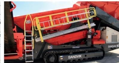
Hydraulically folding maintenance platforms
