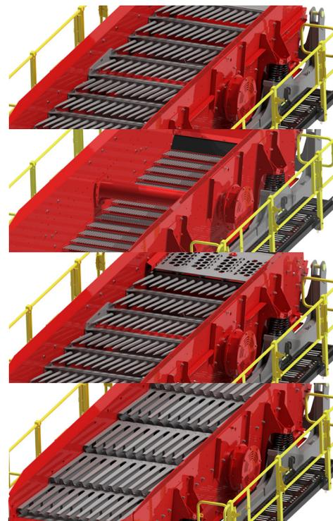
Ability to configure with punch plate, grizzly fingers, bofar bars, mesh or cascade fingers.
